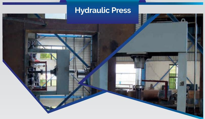
Hydraulic press is also a type of press machine. It uses the hydraulic system to apply force that is used to drive the press. It is used for heavy duty applications where larger force is required as compared to mechanical press. Mainly used for forming with help of dies. We have diverse types of hydraulic presses with different capacities.
