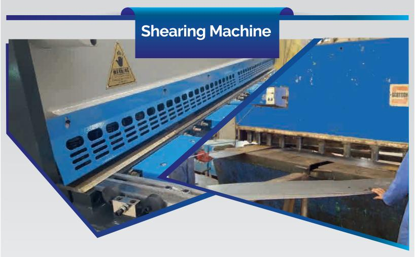
Shearing machines are multipurpose devices used in the cutting of alloys and other sheet metals. It uses a scissor-like action to cut metal into sheets or strips. The machine is hydraulically operated and efficient in shearing of metal.
