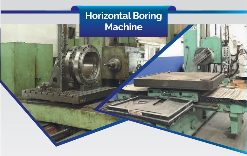
Horizontal boring machine is a time-saving machine used to bore holes in highly rigid construction like machine bodies and gearboxes. A variety of operations can be carried out with the help of this machine-like surface milling, drilling, reaming, boring, turning and facing with the tool held in the facing head slide.
