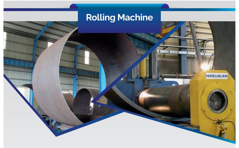
Rolling machine is used to roll a metal sheet or strip. A metal stock is passed through one or more pairs of rolls moving in the same direction that roll it into a curved sheet. We have diverse types of rolling machines with different capacities.
