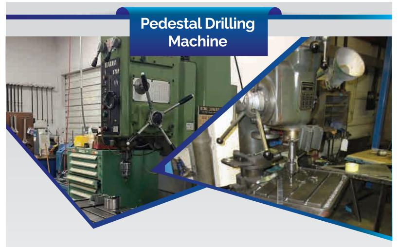
The larger version of the machine drill is termed as Pedestal or Pillar drill. This contains a long column that stands on the ground. The pedestal drill gives a number of benefits over a hand held drill, Controlled amount of pressure using a rotary feed handle, ability to hold the project at hand in place, and precise angle drilling a perfect 90° perpendicular holes in thicker material or precise angles by tilting the table.
