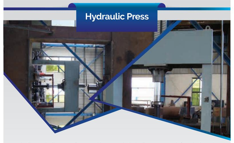
Hydraulic press is also a type of press machine. It uses the hydraulic system to apply force that is used to drive the press. It is used for heavy duty applications where larger force is required as compared to mechanical press. Mainly used for forming with help of dies. We have diverse types of hydraulic presses with different capacities.
