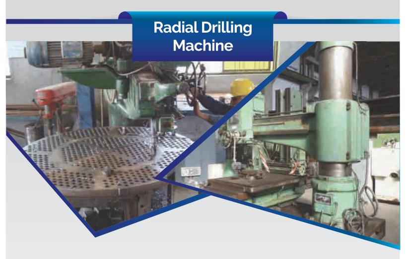
A radial drilling machine or radial arm press is a geared drill head that is mounted on an arm assembly that can be moved around to the extent of its arm reach. The drill head of the radial drilling machine can be moved, adjusted in height, and rotated. We have diverse types of radial drill machines depending on their capacities.
