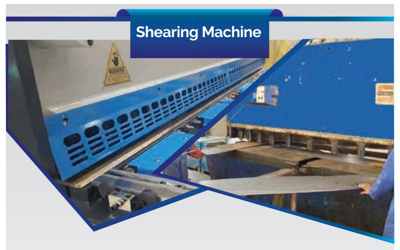
Shearing machines are multipurpose devices used in the cutting of alloys and other sheet metals. It uses a scissor-like action to cut metal into sheets or strips. The machine is hydraulically operated and efficient in shearing of metal.
